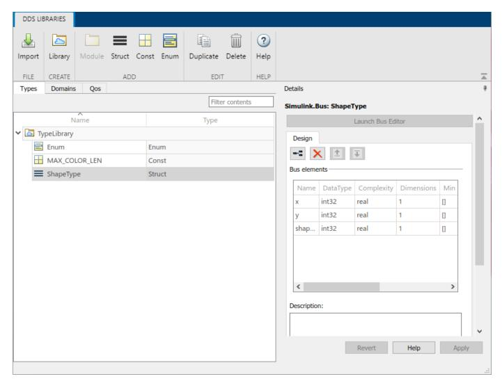
Alternatively, you can open the DDS Dictionary from a Simulink data dictionary. In a Simulink data dictionary, if DDS definitions are available, a **DDS Libraries** node appears in the dictionary. If you open the **DDS Libraries** section of the Simulink data dictionary, in the **Details** pane, you can click **Open DDS Libraries** to open the graphical interface for the DDS Dictionary.
