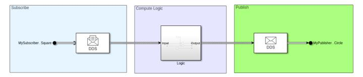
In the Simulink model for the Shapes Demo, view how the DDS blocks, Take DDS Sample and Write DDS Sample, are used to subscribe to and publish the location of the shape.
