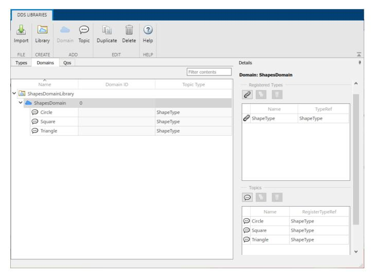
Alternatively, you can open the DDS Dictionary from a Simulink data dictionary. In a Simulink data dictionary, if DDS definitions are available, a **DDS Libraries** node appears in the dictionary. If you open the **DDS Libraries** section of the Simulink data dictionary, in the **Details** pane, you can click **Open DDS Libraries** to open the graphical interface for the DDS Dictionary.
