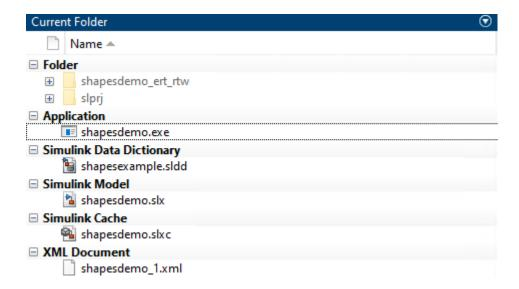
You can use these generated files to analyze, deploy, and port your DDS application. Additionally, you can use the packNGo functionality to relocate and rebuild your application.
