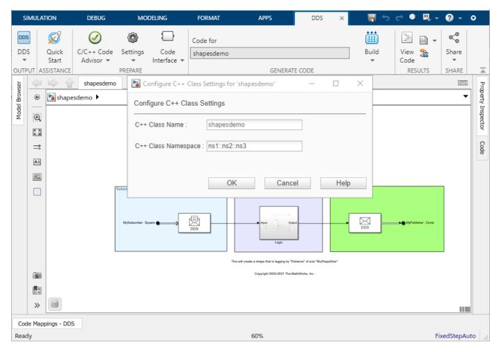
To programmatically configure the class name and class namespace, use the Embedded Coder API functions getClassName, setClassName, getClassNamespace, and setClassNamespace. For more information, see Configure class namespace (Embedded Coder).
